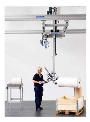
Electric Mechlift is an ergonomically designed moment absorbing lifter that has a stepless frequency steered lifting speed that is controlled via joystick. Mechlift is available in different standard sizes for loads from 75 kg to 650 kg and has a maximum stroke of 2000 mm.
