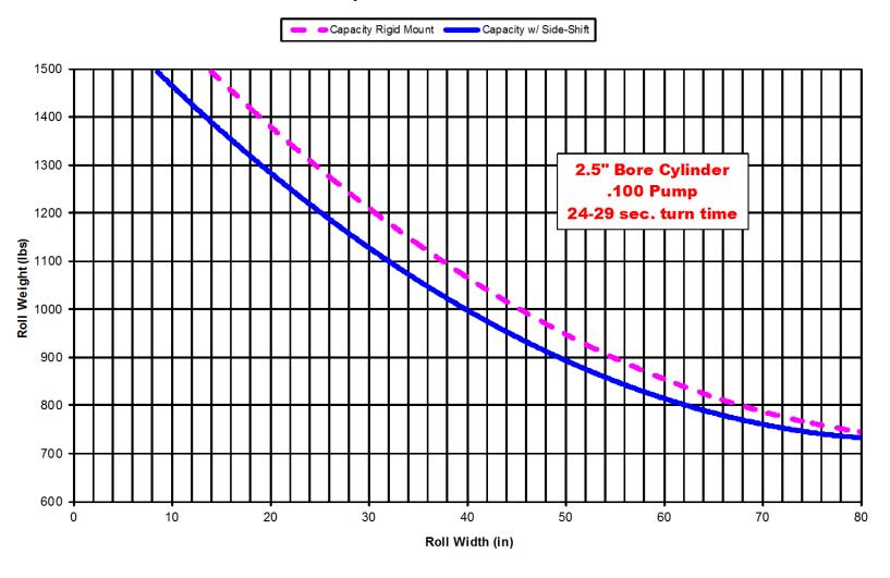
Note: Consult with R&D Ergo before handling rolls heavier than 1000lbs (454kg) or wider than 70" (1778mm).
