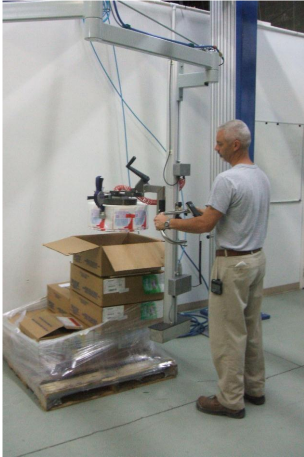
End-Effector Mounted on Mobi-Lift™
