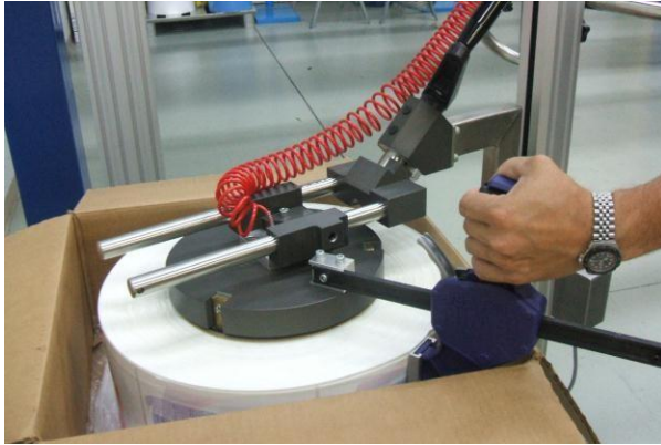
Expand-O-Turn® Inserted into Core with Anti-Telescopic Device Activated
