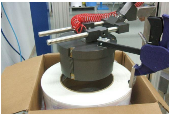
Expand-O-Turn® with Anti-Telescopic Device Pick From Carton Application-10" Core Shown
