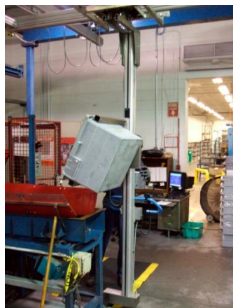
Tote Dumping into Hopper
