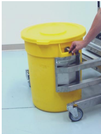
Retaining Pins Installed
