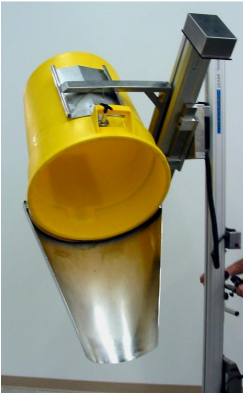
Close Up Showing Chute and Retaining Brackets
